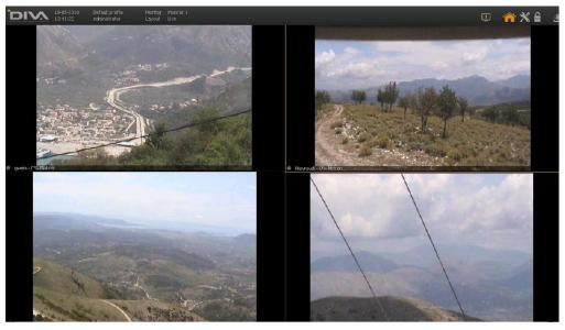
consist of two basic components: a sub-system of 4 cameras that enables people in the operation center, which is located in the building of the Regional Unit, to observe a big area covered with forest and a GIS system, used to produce thematic and fire risk maps. The project was co-financed by national and E.U funds.
