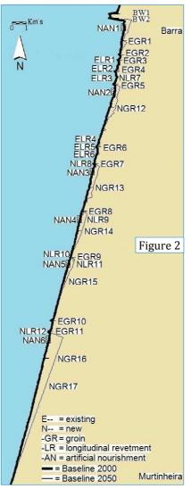
tween extending existing (E--) and establishing new (N--) coastal protection interventions (see Figure 2 for specific locations).
